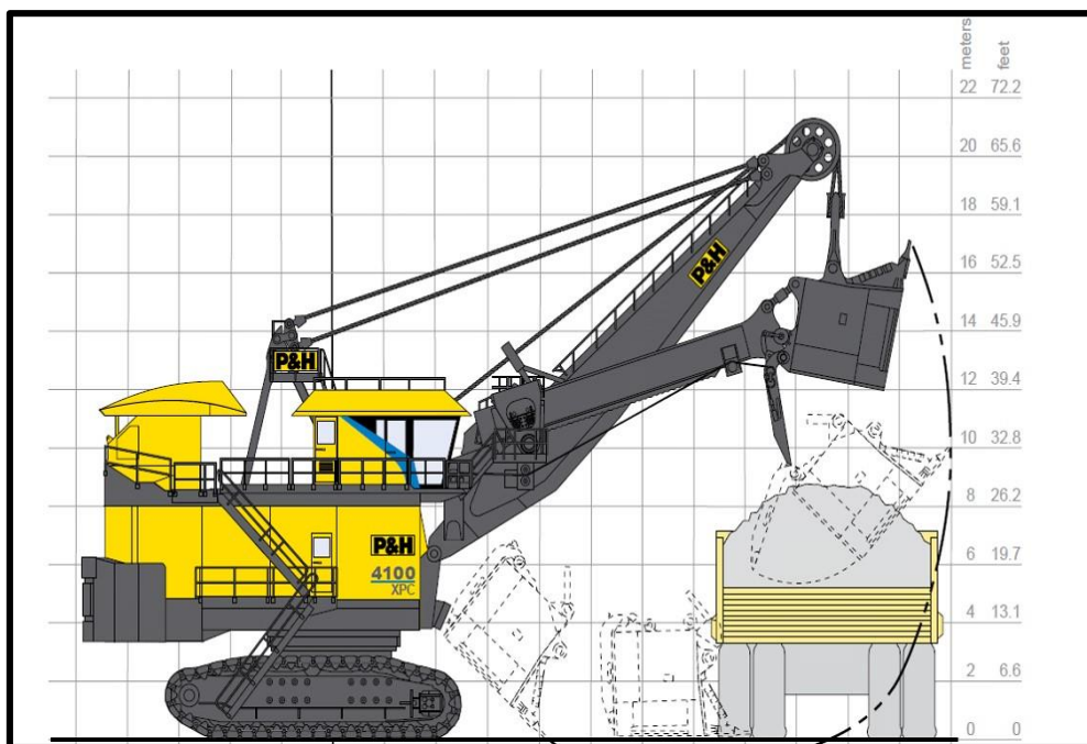
Figure 5.2. Engineering Sketch for P&H 4100XPC Shovel
